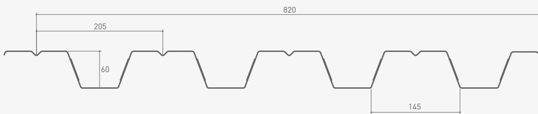
Image 1 – Geometry of H60 profile
